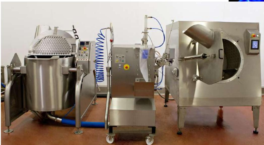
Basic cook-chill arrangement - Ready-2-Cook Kettle, Pump Fill Station, Tumble Chiller.
