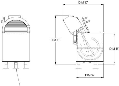
CAN BE ADJUSTABLE FOOT, LOAD CELL PLATE OR TO SUIT CUSTOMER INSTALLATION
