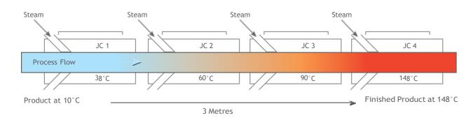
Multi In-line System consisting of 4 Jet Cooks - liquid product taken from 38°C to 148°C in a single pass at flow rates of up to 1000 litres per hour.
